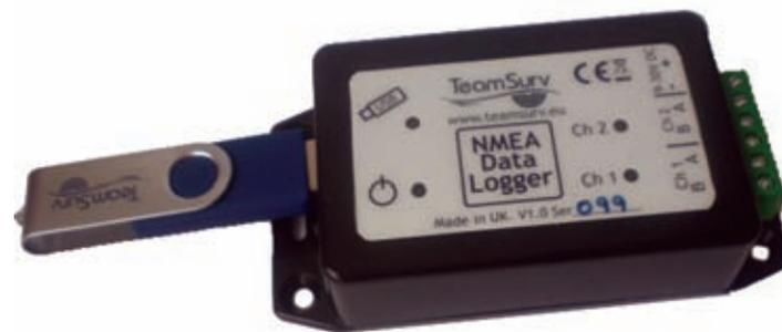
TeamSurv asks mariners to log depth and position data while at sea before uploading it to the web
