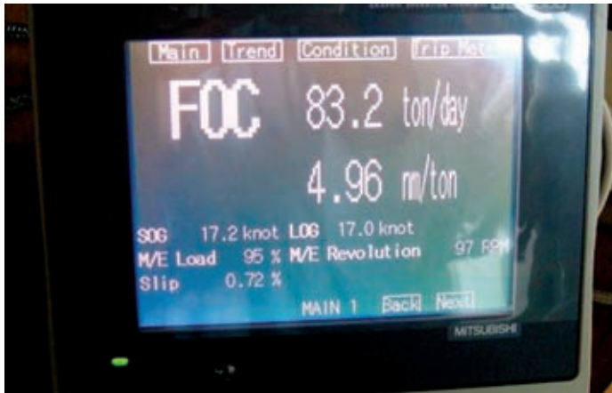
The FuelNavi system collects information from around the vessel, and uses it to display updated fuel consumption levels
