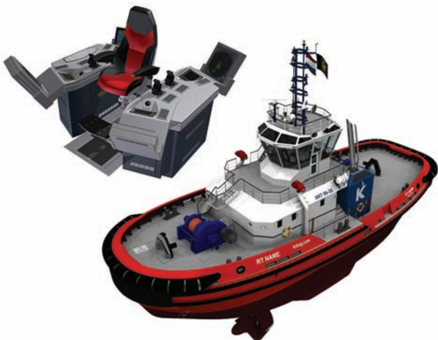
The bridge setup includes ECDIS and Radar in the fore position, with additional multifunction screens for other data
