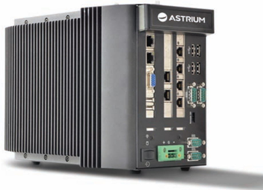
Astrium's XChange box will be used to manage the onboard networks
