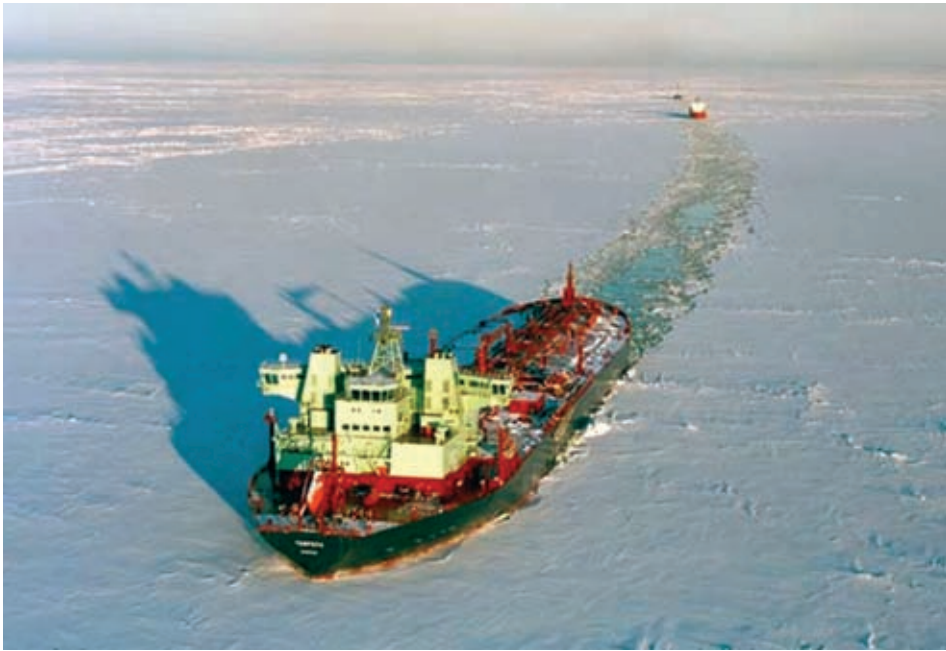
MT Tempera is a double acting tanker (DAT) capable of breaking through thick layers of ice
