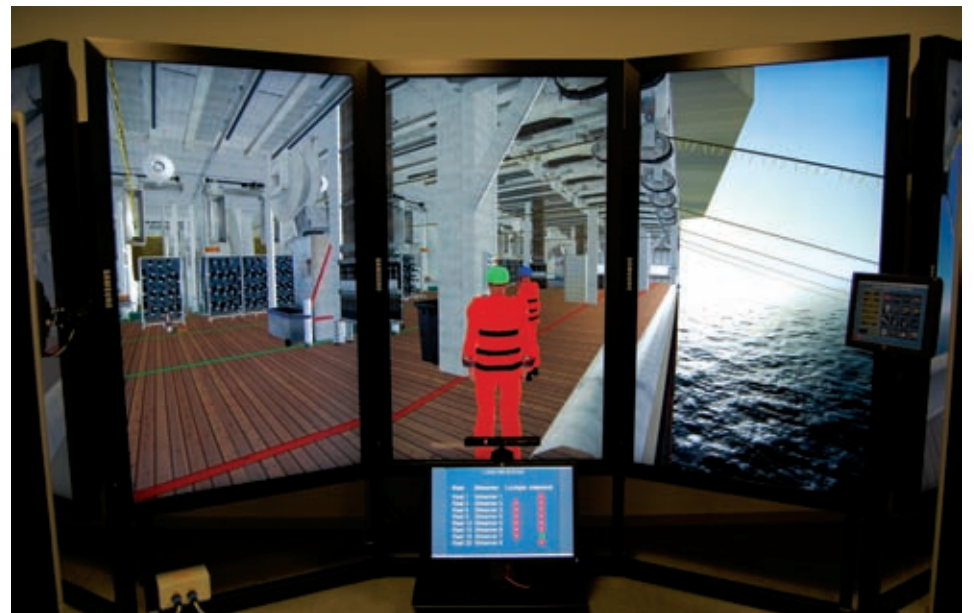
The Kinect technology detects trainee movements and depicts them within the simulated environment
