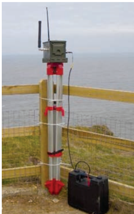
A GPS jamming unit used in trials by the General Lighthouse Authorities, which caused GPS receivers to report position errors of more than 20km. Photo: GLA
