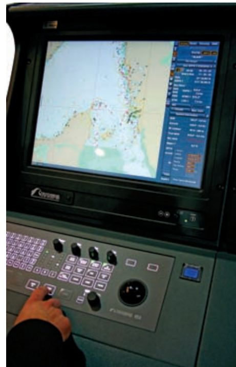
If additional GIS information obscures ENC data on the display then the system can no longer operate as a compliant ECDIS
