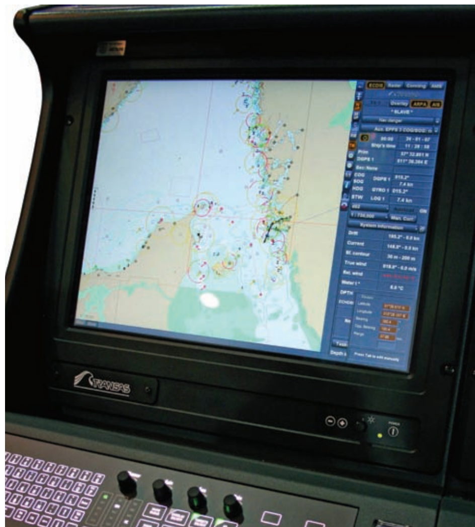
One of the major benefits of using ECDIS is chart updating, which can save hundreds of hours per year when compared with paper charts
