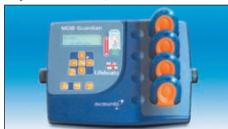
RNLI's man overboard system - sends ship location information by satellite
