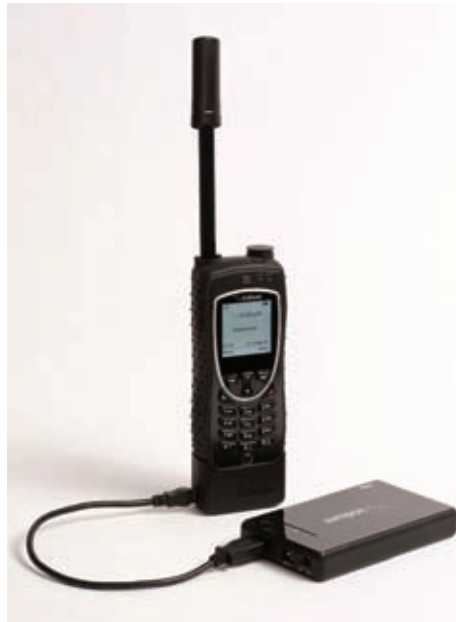
The AccessPoint can turn an Iridium phone into a Wi-Fi hotspot
