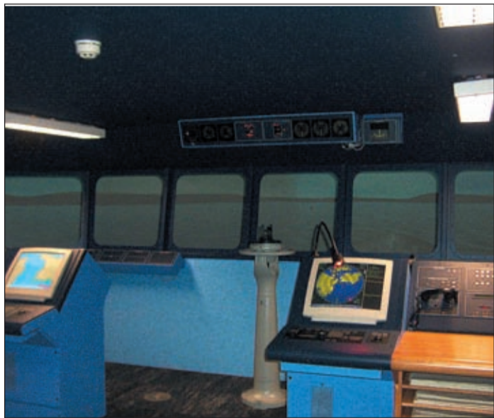
A 270° full bridge simulator - training in virtual reality
