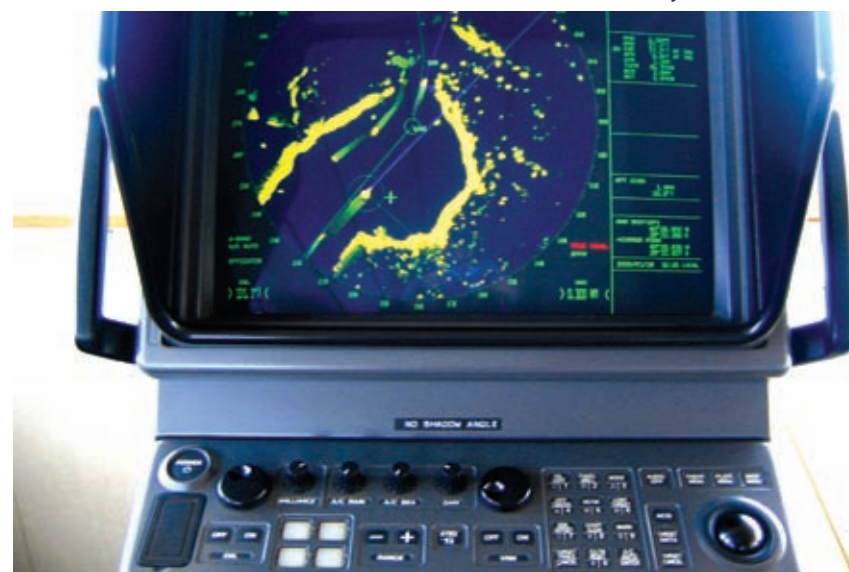
ARPA radar used to be the most complex navigation equipment on the bridge – those days are long gone. Photo: Clipper
