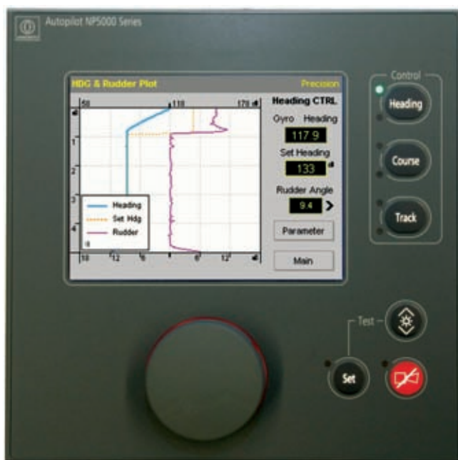
The autopilot aims to optimise rudder movements
