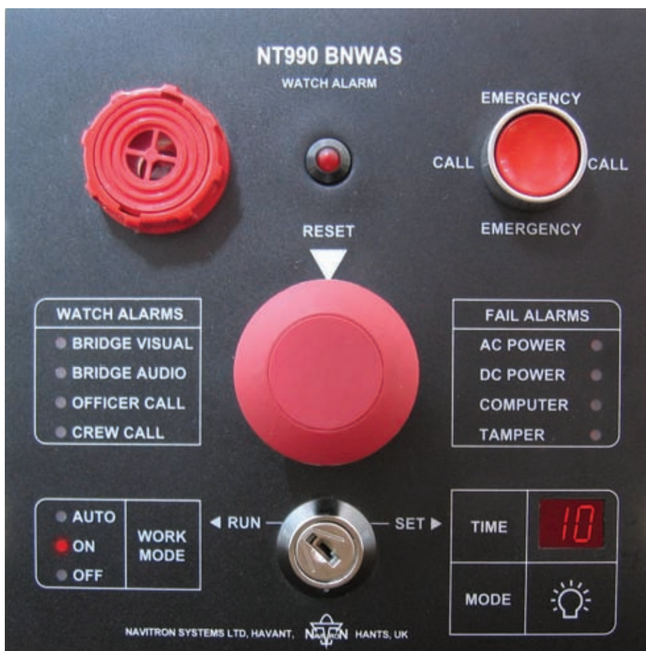
BNWAS requires operators to acknowledge an alarm at regular intervals, for safety purposes
