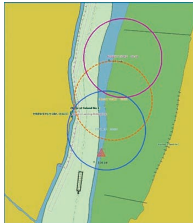
CEACTION can calculate CPA on river miles, route or open sea
