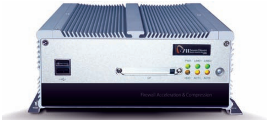
The smart@sea gateway unit will be used to manage communications traffic over the FleetBroadband 500 systems on the ships
