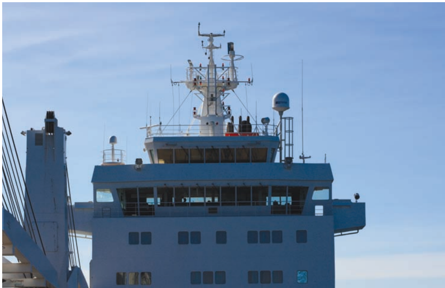
Spliethoff's ships will be installed with the Connector by Radio Holland VSAT service (right), with FleetBroadband (left) as a back-up
