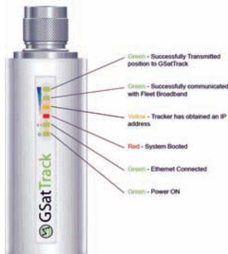
Indicator lights on the unit display the status of the tracking system
